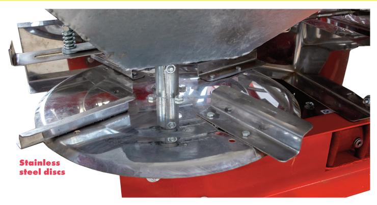
The new MTL – MAXI spreader has evolved with a stronger chassis design to suit heavier loads for larger quantities of fertiliser. The design has been CAD optimised to ensure that the MAXI spreader is very compact, strong and light.
