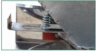
The spread rate adjustment with its shutter slides is located well out of the 'dirty area' meaning that it is not splashed by the tractor wheels or with fertiliser dust from the spreading discs, meaning the machine stays clean and easy to operate. The spreading shutters are opened and closed either by the manual control lever or by the hydraulic ram.
