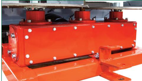
The oil-immersed gearbox is built at the heart of the Junior twin disc spreaders. Double sealed, and with shear bolt overload protection on the 540rpm PTO drive, Junior gearboxes are well proven and are maintenance-free.
