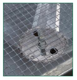
The galvanised in hopper grid is useful when filling with bulk stored fertilisers, as any stones or lumps are stopped from blocking the apertures.
