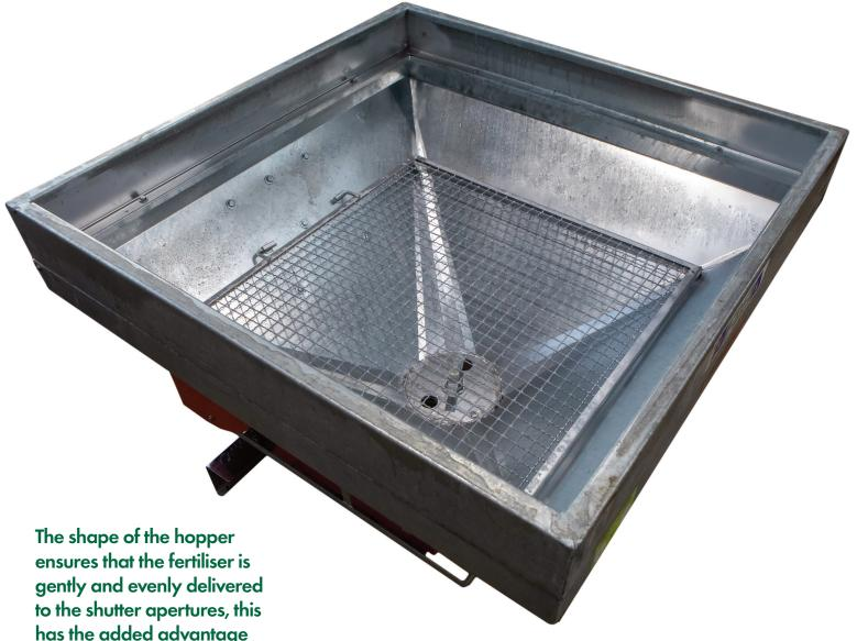
The shape of the hopper ensures that the fertiliser is gently and evenly delivered to the shutter apertures, this has the added advantage that the hopper is virtually completely emptied so there is next to no fertiliser wasted when cleaning the machine out.
