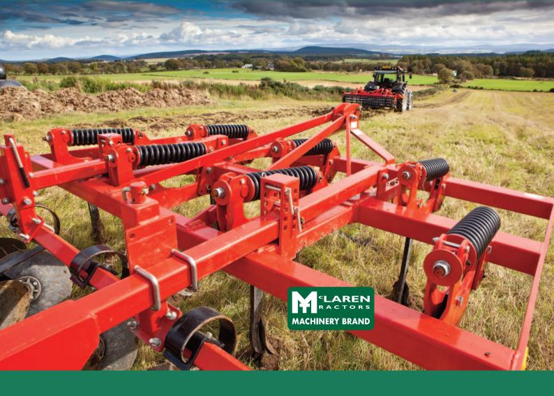
The McLaren Tractors (MTL) Stubble Cultivator has been developed with lightly curved guide plates, mixing the flow of earth from the side – an intensive rolling movement without throwing earth up onto the frame. Also, the outer tines are fitted with edge guide plates.
