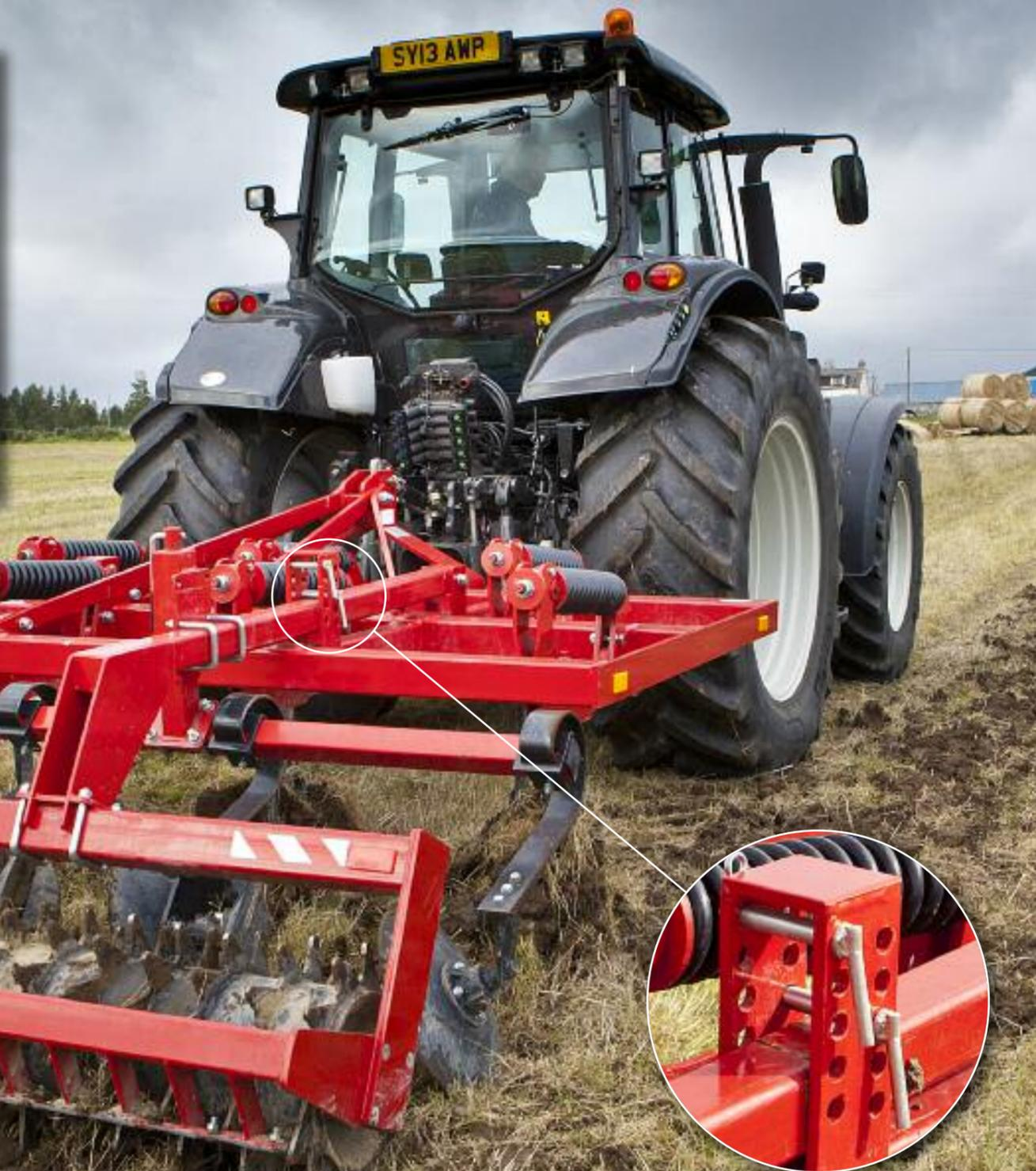
The McLaren Tractors (MTL) Stubble Cultivator has been developed with lightly curved guide plates, mixing the flow of earth from the side – an intensive rolling movement without throwing earth up onto the frame. Also, the outer tines are fitted with edge guide plates.
