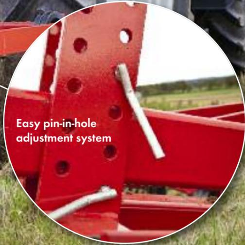
Easy pin-in-hole adjustment system
